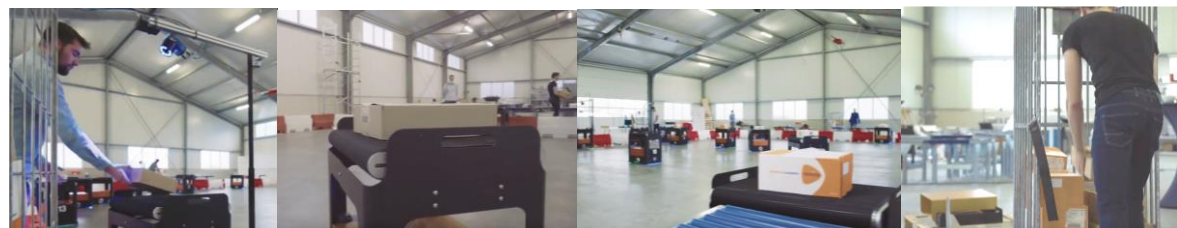
1. The operator scans the parcel and puts it on the Rover 2. The Rover finds its way 3. The Rover drops the parcel at the destination conveyor belt 4. The operator takes the parcel from the roller belt.
