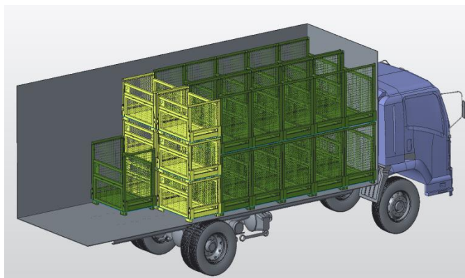
Figure 10. Improved stackability of foldable PI grid boxes
