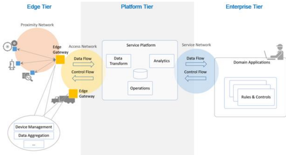
Figure 52: Three-tier system architecture
