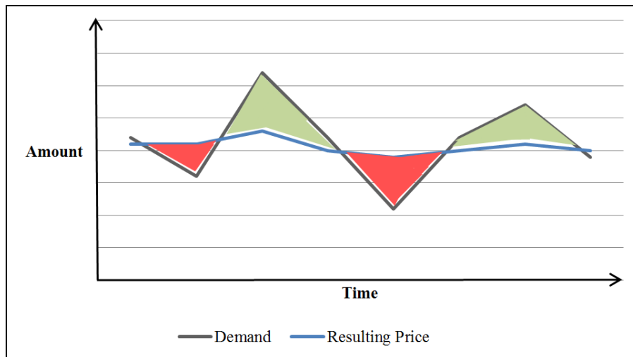
Figure 3: Principle of Equalization by Postponement
